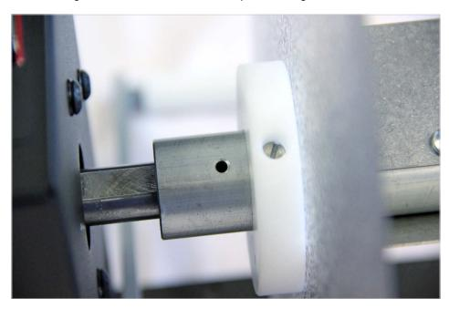
Slide the guide disc so the screw is over the hole and tighten the screw to secure in place. Push the main spindle onto the top shaft as far as it will go.
