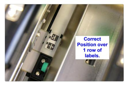
**Note:** When there is more than a single row of labels, the sensors only needs to be over one row of labels and not all of them. For round, oval and irregular shaped labels the sensors needs to be over the narrowest point between labels.
